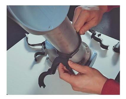
**Step 5-** Repeat this process and install the second Gripping Clamp / LSDFB assembly.
