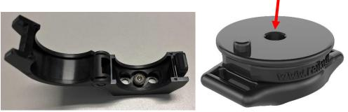
**Step 2**- Place the Gripping Clamp / LSDFB strap assembly against the Cobot arm in the general vicinity that the cables and hoses are to be routed.
