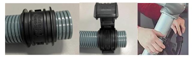
**Step 7**- After you have cycled the Cobot and cut the conduit to length if necessary, insert the 2 supplied PEDST Sealing Caps as this will create a smooth radius edge. Now install your cables and hoses.
