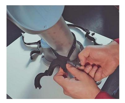
**Step 4**- Once the Gripping Clamp / LSDFB are securely held in place against the Cobot arm engage the Velcro surfaces to lock the assembly in place.
