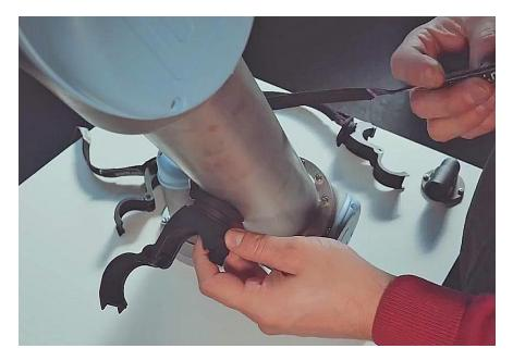
**Step 3**- Loop the end of the Velcro strap through the slotted opening in the rear of the LSDFB and pull forward until all the slack in the strap has been removed and then wrap around the Cobot arm.
