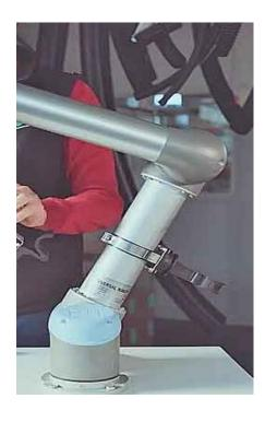
**Step 4-** Repeat this process and install the second Gripping Clamp / MESUB assembly onto the upper Cobot arm in the general vicinity that the cables and hoses are to be routed and then tighten securely.
