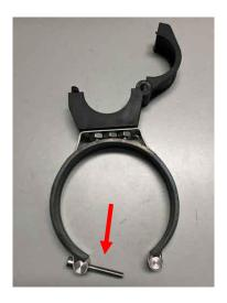
**Step 3**. Place the assembly with the larger diameter MESUB metal strap around the lower/base Cobot arm in the general vicinity that the cables and hoses are to be routed and then tighten securely.
