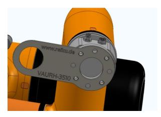
**Step 9**- Insert the REIKU conduit connector into the hole in the "Frying Pan" with the threads facing away from the CoBot and secure with the supplied locknut.
