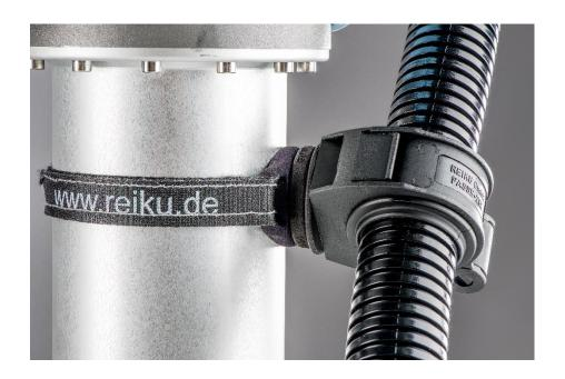
**Step 1**- Secure the PASSB Style Gripping Clamp (with the screw provided) to the mounting hole in the centre of the LSDFB "turntable".
