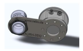
**Step 10**- Insert the REIKU conduit into the connector and install cables and hoses.
