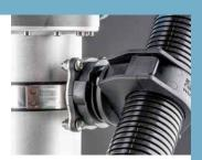
**LSDFB:** Suitable for easy use at cobots with slow to average movement speeds and low loads. Usually, LSDFB items are passed NW17 to NW29. The console of LSDFB is attached to the robotic arm to prevent it sliding and the turntable allows variable cable management.
