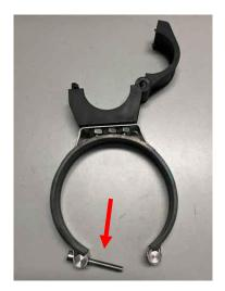
Step 3. Place the assembly with the larger diameter MESUB metal strap around the lower/base Cobot arm in the general vicinity that the cables and hoses are to be routed and then tighten securely.
