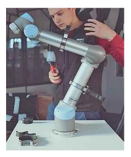
\*An additional third clamp assembly can be added to the upper Cobot arm for heavier conduit loads or for applications that involve high dynamics.
