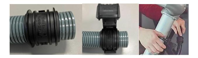
Step 7- Insert the supplied PEDST Sealing Caps into the conduit end which is at the base of the Cobot as this will create a smooth radius edge.
