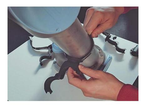
**Step 5-** Repeat this process and install the second Gripping Clamp / LSDFB assembly.
