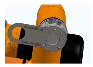
Step 9- Insert the REIKU conduit connector into the hole in the "Frying Pan" with the threads facing away from the Cobot and secure with the supplied locknut.
